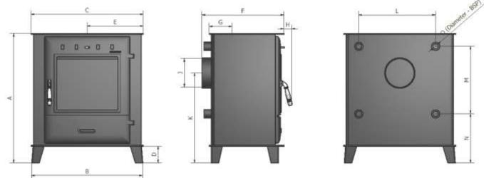
Fig 1 – Causeway 16 and Causeway 25 boiler stove dimensions
