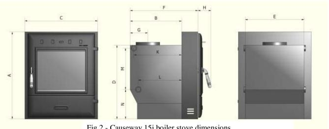
Fig 2 - Causeway 15i boiler stove dimensions
