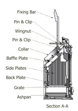
Fig 2 – FW5i Stove Assembly and controls
