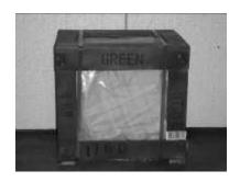
Carefully remove the steel straps and lift off the upper crate.
