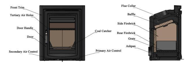
Fig 2 – Stove Assembly and controls
