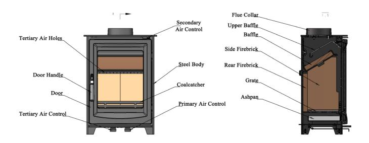
Fig 2 – Stove Assembly and controls
