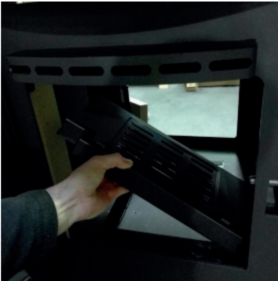
2: Remove the log guard and cast iron grate - care should be taken to avoid damaging the vermiculite bricks.
