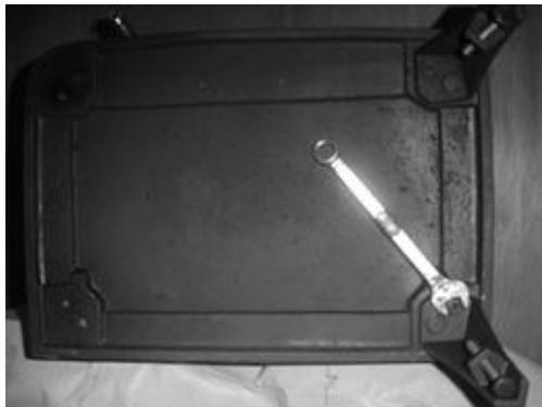
**1. Fit the Flue Collar using the 4-M6 set screws and washers supplied. Screw The M6 nuts on the M6 screws all the way to the end. Then put the washer over the screw/nut assembly and secure the collar to the lid/back as desired.**
