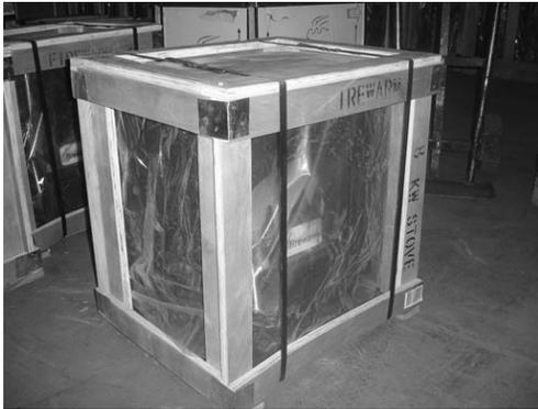
Carefully remove the steel straps and lift off the upper crate
