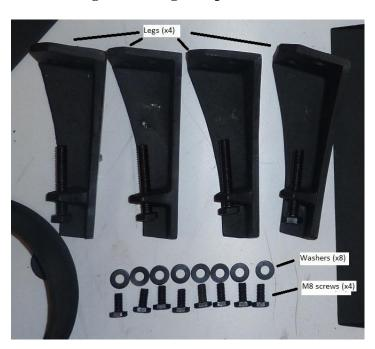
3. Ensure the tapped holes, on the base, are free from obstruction. Use a sharp screwdriver to remove any fire cement. Secure the legs and fixings using the screws and washers provided, two screws and two washers per leg.
