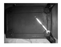
5. Ensure the tapped holes, on the base, are free from obstruction. Use a sharp screwdriver to remove any fire cement.
